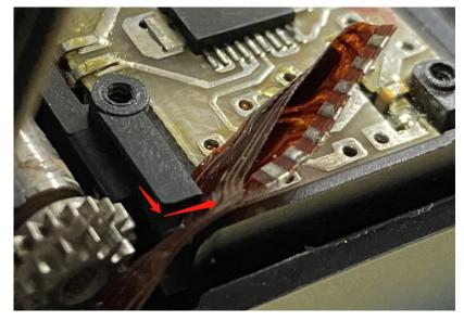
Step3: Pins to be desoldered:
