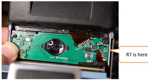
**Step7**: Solder the flex cable which connect the body and ECM. Then PLEASE DEFINE YOUR CAMERA MODEL, FOR SLR680 YOU HAVE TO <u>REMOVE R7</u> to disable the fill flash function (please pull out the battery before you do this) you don't have to do this on a Sonar (this note added after June 18, 2024)
