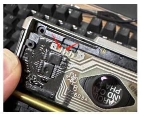
Step3: Does the flash fire? Fired—Set A, Not fired—Set B (showed as below)
