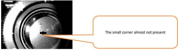
• For a MODEL 1 camera, after the calibration the small corner should not be present:
