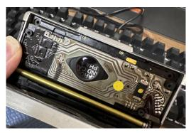
**Step2:** Insert a flash like MINT Flash Bar, when flash **ready**, short two pins show below with a metal tweezer, that is, the first pin and the second pin of FFA
