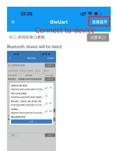
Connect to the device with "CH9141BLE2U", it's the name of the camera default.
