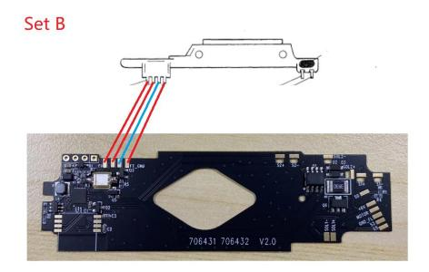
**Step6:** For other pins, re-press the pins, then solder them as they soldered on the old boards before. And please solder them firmly, as shown in the photo below, which is a comparison image after removing the old circuit board and installing the new one, please pay attention to Step3 and ensure reliable solder joints and no adhesion. If it is a 4-pin solenoid, it needs to be converted into a 2-pin solenoid, please refer to the operation in the appendix.
