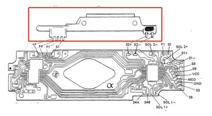
So, before installation, you need to confirm the type of FFA, otherwise it will cause failures such as failure to trigger the flash. There are three types of FFA: high-voltage trigger type, low-voltage trigger type, and thyristor type. You need to confirm the FFA type before installing the circuit board. Here are how to do:
