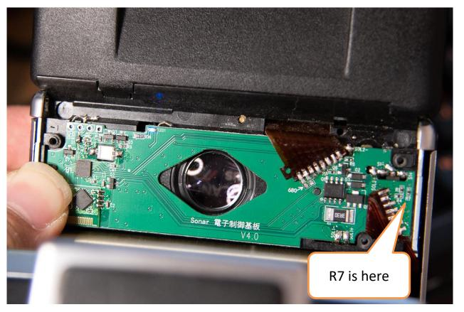
**Step7**: Solder the flex cable which connect the body and ECM. Then PLEASE DEFINE YOUR CAMERA MODEL, FOR SLR680 YOU HAVE TO <u>REMOVE R7</u> to disable the fill flash function (please pull out the battery before you do this) you don't have to do this on a Sonar (this note added after June 18, 2024)
