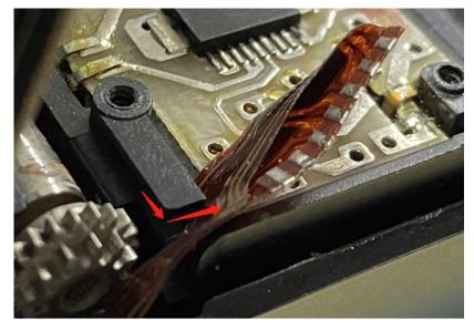
Step3: Pins to be desoldered:
