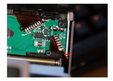
**Step8**: Apply a black tape used for covering the back side of the sensor, to prevent the light from the back side of the camera.
