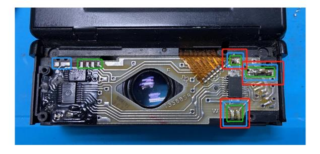
Note: The pins need to be desolder and pull to a vertical position and separated from the solder pad.
