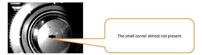
• For a MODEL 1 camera, after the calibration the small corner should not be present:
